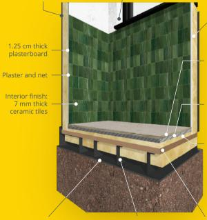
0.5 mm thick, anti-corrosion treated galvanized sheet 150 mm C profile
